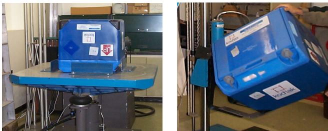
Vibration and Impact Load Testing Taking Place
